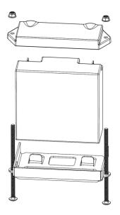
**Why:** To reduce the possibility of fertilizer contamination and build up on the Gateway battery post(s), Stinger developed a custom fit battery cover (included) and hardware kit.
